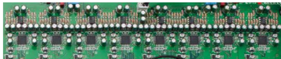
D/A converter circuit Extensive use of high quality parts - *MUSES 02* Op Amp, AKM *AK4495S* DAC chipset, etc.
