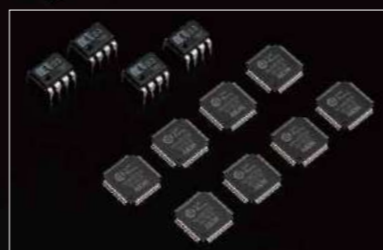
Extensive use of high quality parts (AK4497 DAC IC, MUSES 03 Op-Amp)
