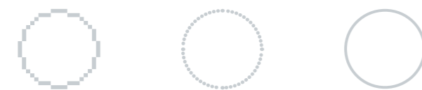
Comparison of a circle in PAL/NTSC, Full HD 1080p and 2160p / 4K x 2K resolution.
