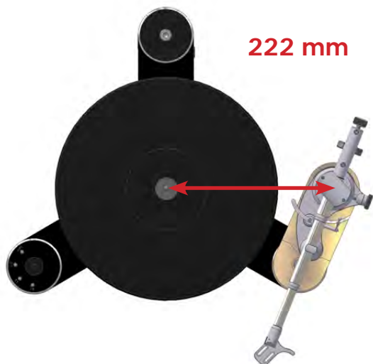
Pic. 5a: Distance from spindle to pivot 222 mm / Universal 9"
