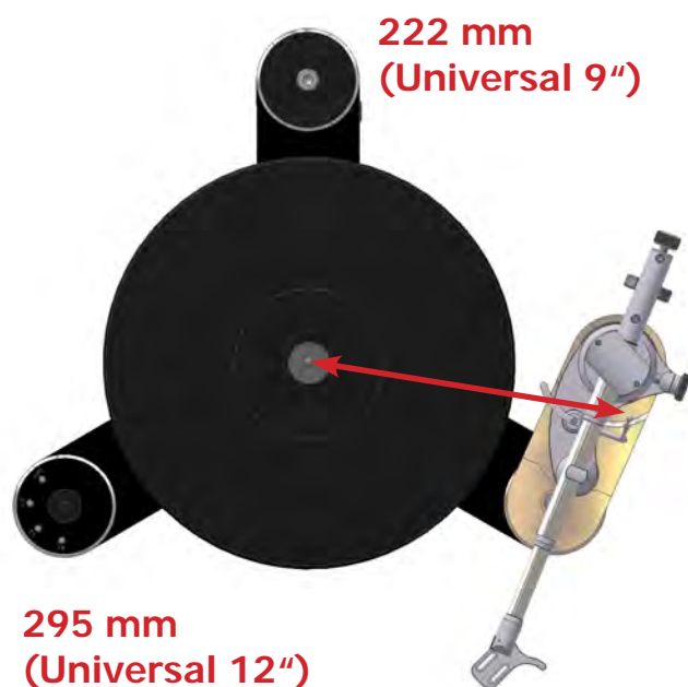
Pic. 8: Distance from spindle to the pivot (222 mm/ 295 mm)
