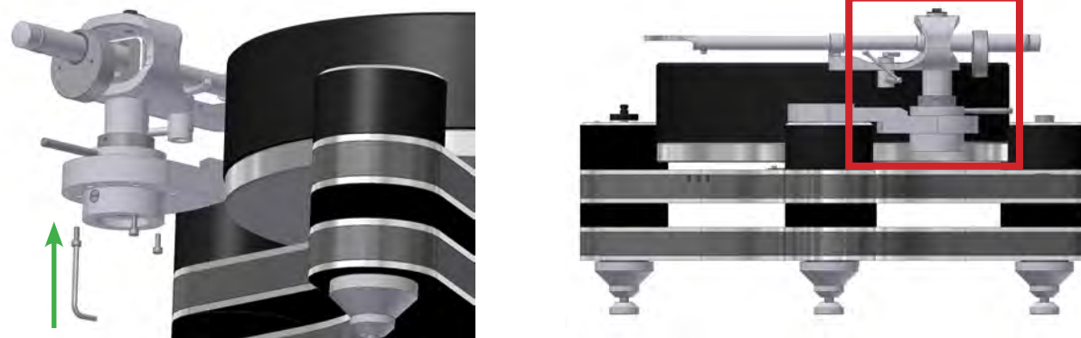
Pic. 3: Set up of tonearm base with VTA-Lifter
