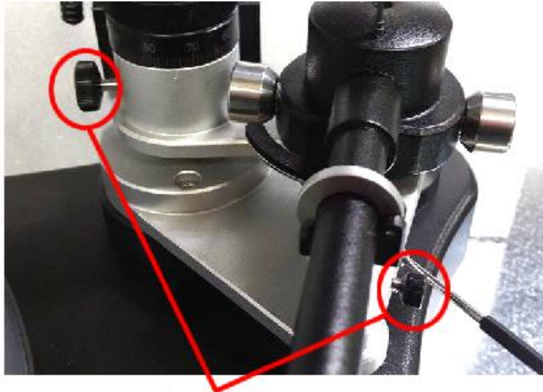
Loosen these two screws to adjust VTA and tighten when set
