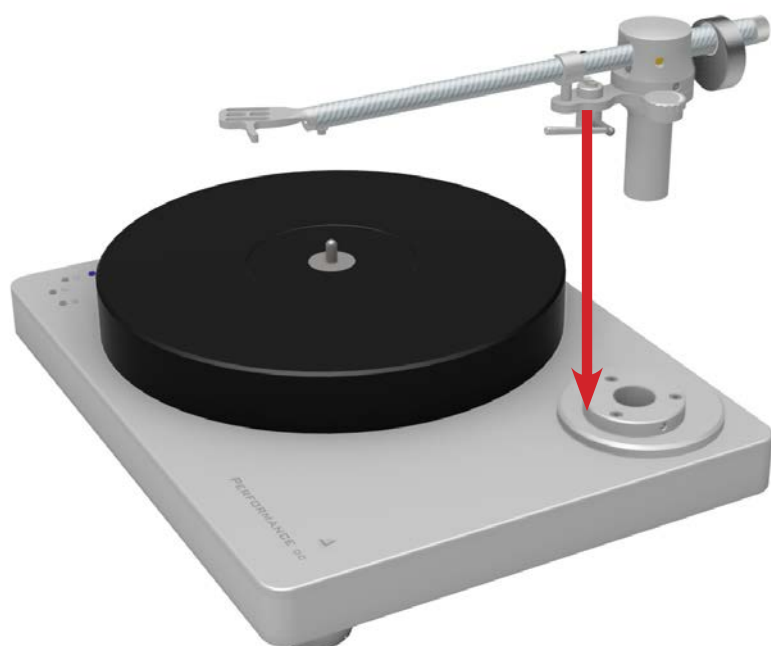
Pic. 3: Threading the tonearm through the armboard
