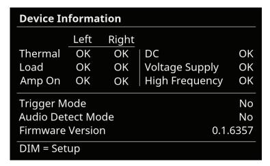
The rear panel on-mode switch positions are shown for reference along with the firmware version and status of various operating conditions. If a fault is detected, a message will appear automatically at the bottom of the power meter display.
