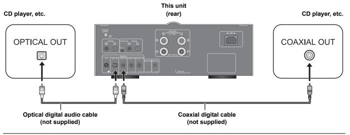
• The digital audio input of this unit supports only the linear PCM (LPCM) signals listed below. For details, refer to the operating instructions of the connected device.
