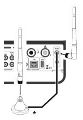
\* The aerial can also be set up free-standing using the magnetic base supplied in the set; this ensures maximum possible range.
