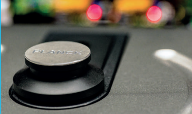
High precision puck and mounting made of POM.
