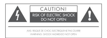
This lightning flash with arrowhead symbol within an equilateral triangle is intended to alert the user to the presence of non-insulated "dangerous voltage" within the product's enclosure that may be of sufficient magnitude to constitute a risk of electric shock.
