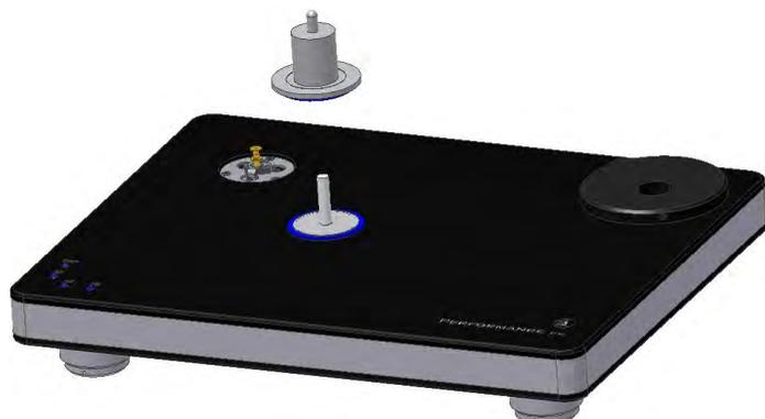
**Pic. 6:** Fitting the bearing upper part
