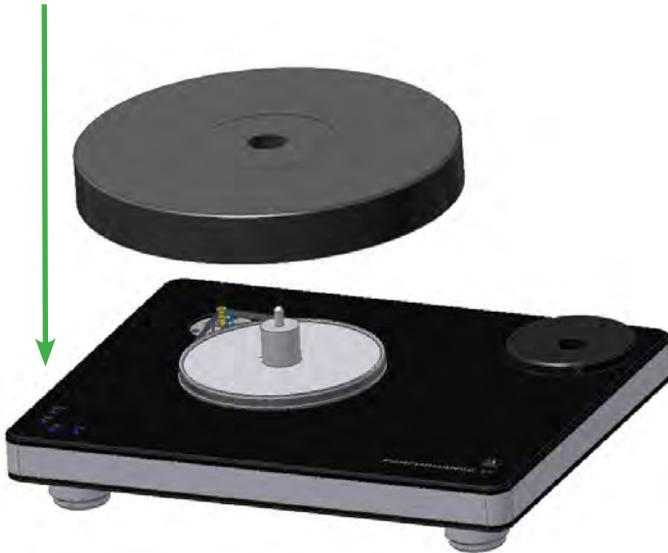
**Pic. 8:** Setting the platter onto the bearing
