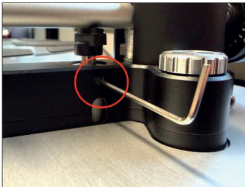
Fig. 14 Height adjustment of the lift bench.
