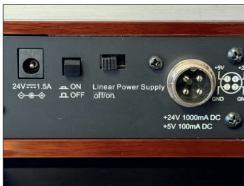
Fig. 20 Connection terminal for power supply.
