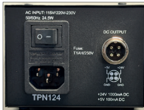
Fig. 18 Connection of the TPN 124 linear power supply.
