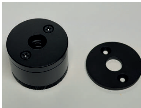
Fig. 6 Counterweight with one additional weight attached and the second additional weight.
