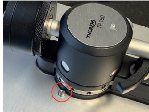
Fig. 24 Adjustment screw for the limit switch.
