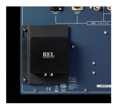
Loosen and remove the two lowest fasteners on along the lower left edge of the amplifier panel. You will need a 3mm hex (Allan) wrench. Then align the holes in the mounting bracket with the holes in the panel. Replace the fasteners and tighten.
