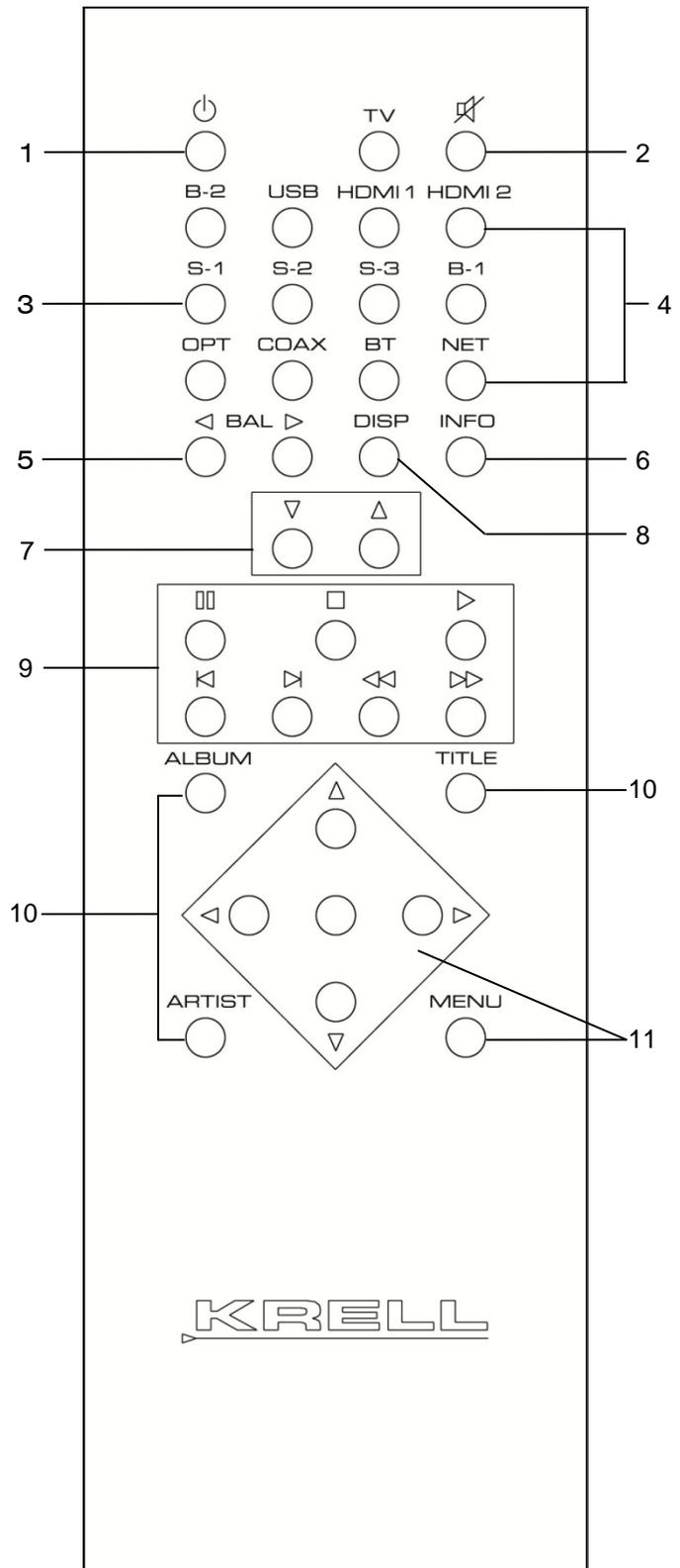
**Note:** The remote comes with two AAA batteries that have to be installed. Use the supplied Torx screwdriver to remove the 4 Torx screws (T10) securing the rear cover then install the batteries.
