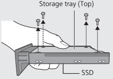
Hold the SSD with one hand to prevent it from falling.
