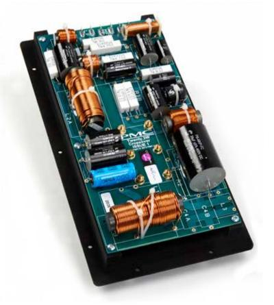
To seamlessly integrate the high, mid and bass drivers of the **twenty.26** takes a highly complex and well-engineered crossover. It ensures the perfect supply of frequencies for each of the three drive units.
