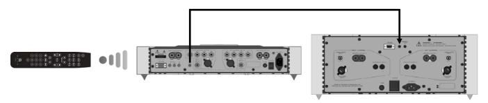
Figure 5: Remote Operation with 12V Trigger
