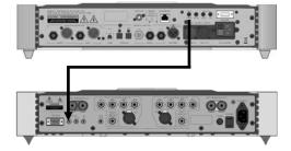
Figure 4: Remote Operation with SimLink™
