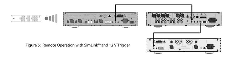
In figure 5 we have a **Nēo 280D** DAC connected to a **Nēo 350P** Preamplifier via their respective SimLink™ ports (using a 1/8″ mini-jack cable), and the **350P** is connected to a **Nēo 330A** Amplifier via their respective 12V triggers (also using a 1/8″ mini-jack cable). When you turn on the **280D** via remote control or by pressing & holding its Standby button, both the **350P** and **330A** will turn on automatically. The same rule applies when you put the **280D** into Standby mode.
