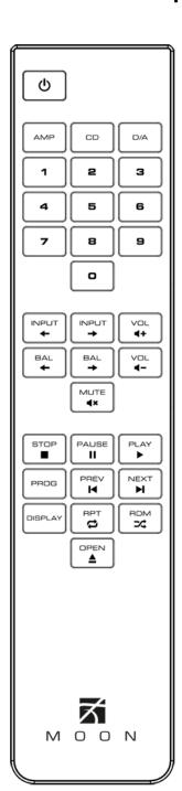
The **Nēo 280D** Digital-to-Analog Converter uses the **'CRM-3'** full-function remote control (figure 6). It operates on the Philips RC-5 communication protocol and can be used with other MOON components.
