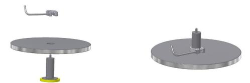
Pic. 5: Connection sub-platter and bearing upper part
