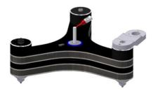
Pic. 4: Oiling the bearing shaft
