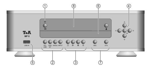
All the important functions of the **MP 8** can be operated using the buttons on the front panel. Direct-acting buttons are provided for fundamental functions. Functions not needed so frequently are controlled using menus which are called up using the **sys** and **src**-button. The following section explains the functions of the buttons on the machine, and the information provided on the screen.
