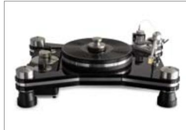
The HR-X features a triple laminated chassis (Acrylic-Aluminum-Acrylic), integral air suspension (which rejects up to 98% of acoustic feedback) and an inverted main bearing incorporating a hardened steel ball running on a Teflon/Delrin composite.
