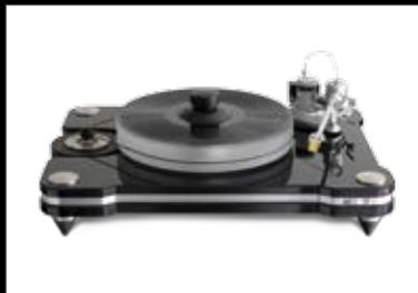
The 1.75"-thick platter is comprised of clear or black acrylic and incorporates an inverted bearing similar to that used in the HR-X. The bearing shaft is 60 Rockwell hardness, ground and polished, and the platter rotates on a Teflon/Delrin composite thrust plate for ultra low noise.
