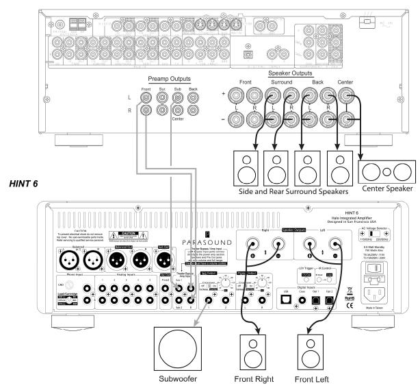
The HINT 6 Bypass Inputs should not be connected directly to any source component with a fixed output level. Examples are CD players, most Blu-ray/DVD players, tape decks or tuners. Since there is no volume control with the Bypass input the full voltage output from the source will go directly to the HINT 6 power amplifier. The sound level could be extremely high and could damage your speakers.
