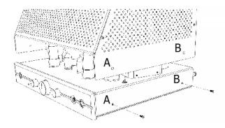
1. Take note of the two screw holes on each side of the SL-100 chassis and the two countersunk holes on each side of the top cover as they should line up properly on both sides before installation.
