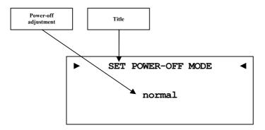
There are two different power-off modes available for the DNP. Firstly the **normal** power-off mode and secondly the **Quick Start** mode.
