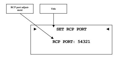
Enter the port number for communication between DNP and the software Audionet RCP or Android app aMM or iOS app iMM. If necessary, you may adjust the port number in a range of 50000 to 59999. The factory default value is 54321. Changing the default value will only be necessary if this port number is already used in your network. If necessary, ask your network administrator for support.
