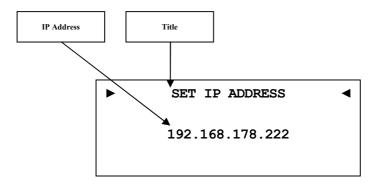
Enter the fixed IP address you would like to assign to the DNP. The IP address type is IPv4 (e.g. 192.168.178.222).
