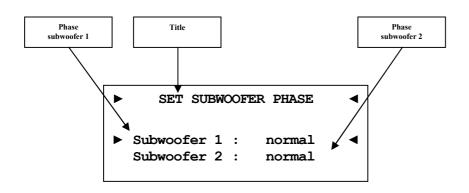
normal0° phase shift.inverted180° phase shift.
