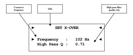
Now you have to adjust the cross over frequency for the speakers. The frequency defines the point of operation for the corresponding filters of your loudspeaker setup. Adjust the Q factor of the current high pass filter. The default setting is 0.71 and should only be altered by experts.
