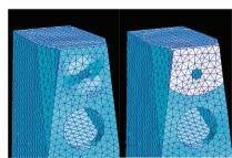
Without plate vs. with plate The diecast aluminum tweeter plate is very effective in damping the vibrations that occur during high frequency output.
