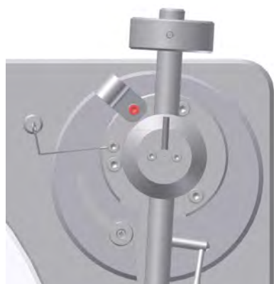
Pic. 3: Placing the arm tube to the pivot point
