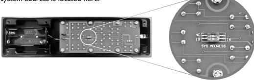
Set the DIP switch labelled 'SYS ADDRESS' to position '19' or '16' according to the following table:
