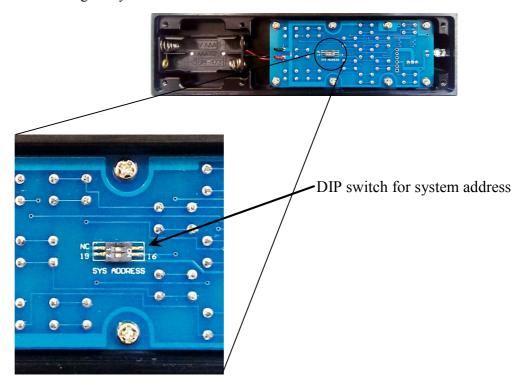
Put the DIP switch labelled 'SYS ADDRESS' in position '19' or '16' according to the following table:
