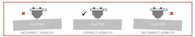
If any adjustment is required, you must first adjust the LEFT to RIGHT and then the FRONT to BACK. See below:
