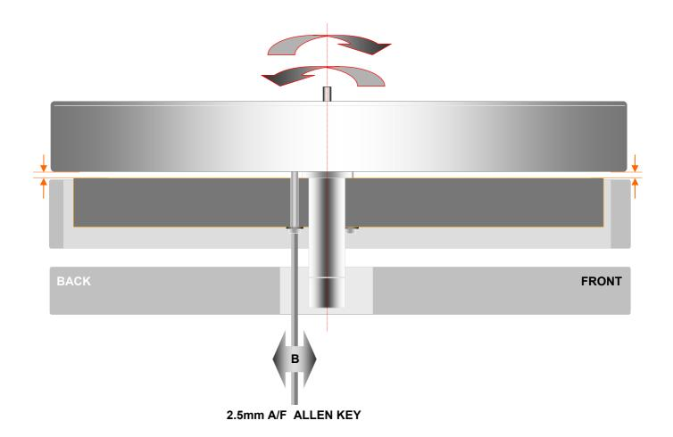
Use the 2.5mm A/F Allen Key and looking from the left hand side, adjust the back (3<sup>rd</sup>) screw to tilt the platter assembly FRONT to BACK as shown above. DO NOT over tighten or slacken the fixing screw too much. Adjustment of this screw will NOT change the LEFT to RIGHT level.
