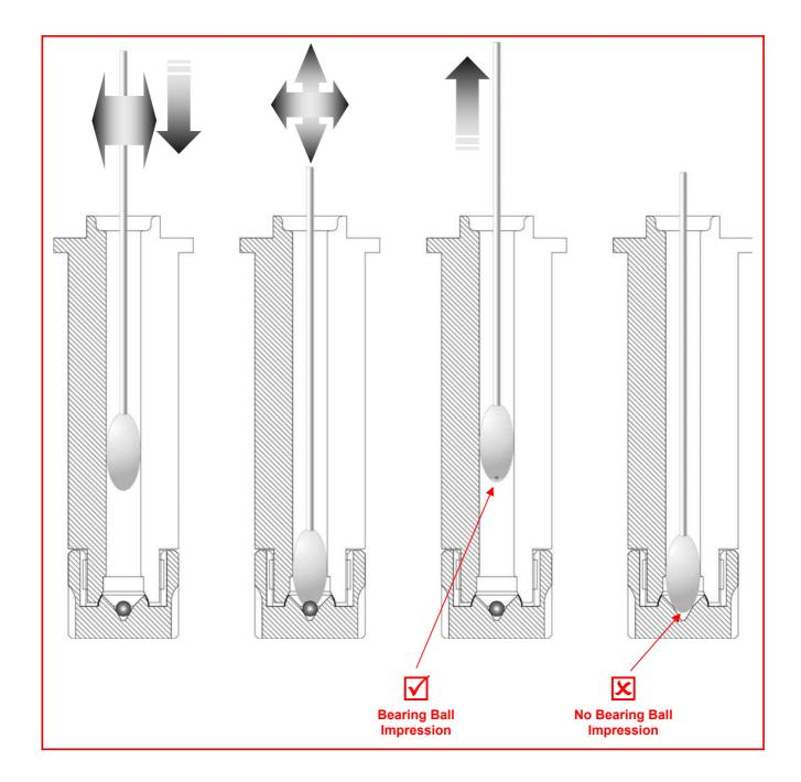
Refer to SETUP section above for detail on charging the Main Bearing with Roksan Supplied oil.
