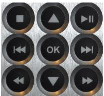
Navigation keys allow you to use the menus. These keys also work to track forward and back, stop, play, pause and also fast forward or fast back any track.
